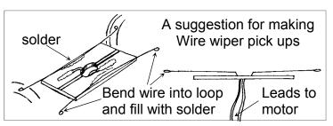
I have also produced comprehensive hints and you are experienced in setting up a chassis. If tips help sheets for using Slater's wheels, etc. These can also be plunger pickups, downloaded free of charge from my website with my motor and gearset. These can be www.jimmcgeown.com or send a SAE and I will be pleased to provide a free copy of my hints and
