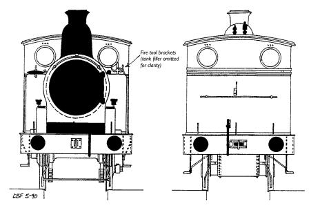
Note alternative boiler fittings and positions. Hole centres are marked on underside of boiler.
